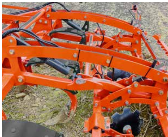
More ease of use offers the parallelogram linkage of the models with the "P". Here the working depth can be changed for the cab on the go.
