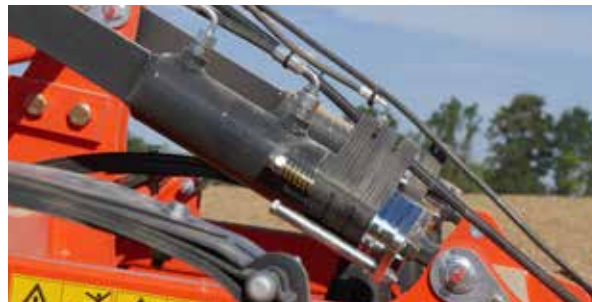
Depth control adjusted with hydraulic cylinder and spacers on CU3001.
