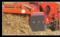
Floating side deflectors with overload protection allow smooth operation and a ridge free soil surface.
