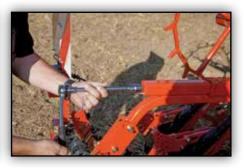
Depending on the soil conditions the pressure and angle of the following harrows can be adjusted manually.
