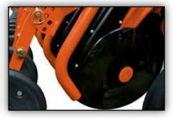
CX-II coulter with double entry for fertiliser application (red tube) and seeding (black tube) in one pass.
