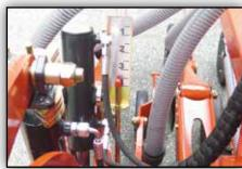
The sowing depth can be adjusted toolless by spacers which are located at the two outer hydraulic cylinders. The operator can see the coulter pressure setting on the scale which is 10 easily visible from the tractor cab.
