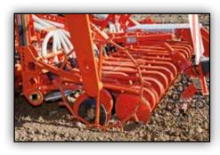
Landwheel with integrated brake to prevent overseeding, e.g. on headlands
