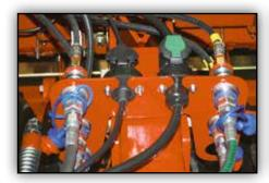
The electronic and hydraulic interface is easily accessible.
