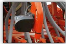
Always the right speed! A radar speed sensor records the speed in order to maintain the relevant distribution rate at the correct time.
