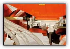
Central position of the metering device with easy access under the hopper.
