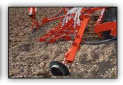
Exact continuation from one tramline to the next is ensured by the use of hydraulically folding track markers.
