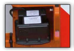
An optional available radar speed sensor can simultaneously record the speed SH1150 in order to maintain the relevant distribution rate
