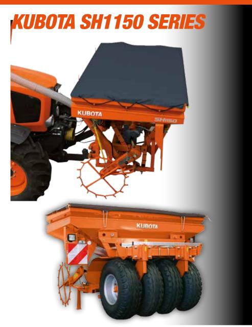
The modular structure of the Kubota SH1150 ensures even weight distribution across the machine arrangement, giving the tractor maximum balance. This improves both safety and manoeuvrability, whilst at the same time giving the driver an unrestricted view over the entire machine set-up.
