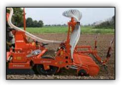
The coulter bar is attached to the harrow via the coulter toolbar linkage. This ensures to maintain a constant seeding depth. The rapid coupling system allows the power harrow to be converted easily for solo use.
