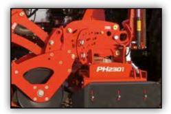
A parallelogram and a quadruple joint of the seeddrills ensure the optimum adjustment of the power harrow and coulterbar for a precise seed application. Important: the adjustment of the power harrow has thus no impact on the coulterbar resp. on the seed depth.
