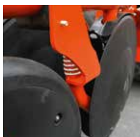
The Kubota CD-coulters consist of two steel discs (Ø410mm) with 12.5cm row spacing. Perfect depth control is ensured by the press wheels (Ø 380mm).
